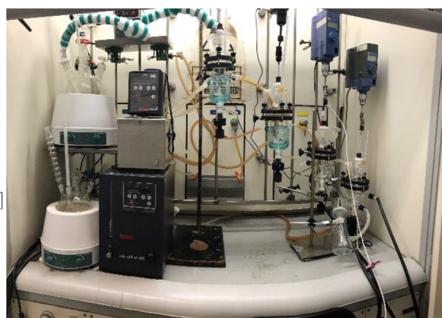
Figure 3. Schematic (a) and photographic (b) illustrations of the continuous crystallizer system.
