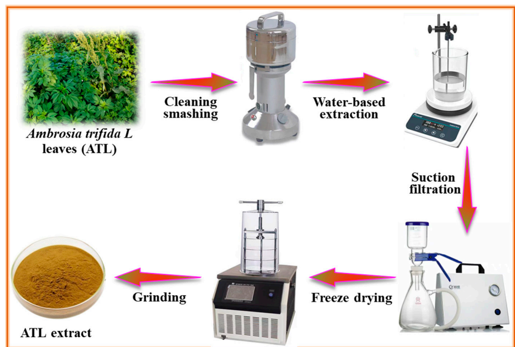
Figure 1. The preparation schematic diagram of the ATL extract.
