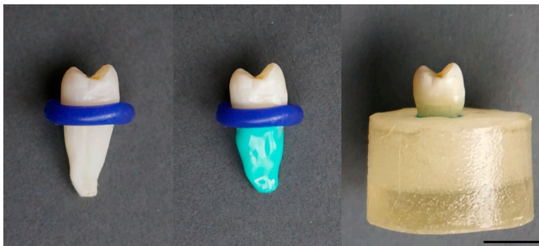
Figure 1. ETT premolar restored with occlusal direct resin composite filling. The enamel–cementum junction was covered by a ring of wax (left). Root surface was coated with A-silicon for simulating the biomechanical behavior of the periodontium (middle). ETT was embedded into transparent resin (right). Scale bar 1 cm.
