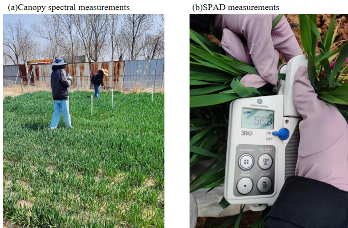
Figure 4. Data Measurements. (a) Canopy spectral measurements using the SVC HR-1024i spectrometer. (b) SPAD measurements with the SPAD-502 handheld chlorophyll meter.
