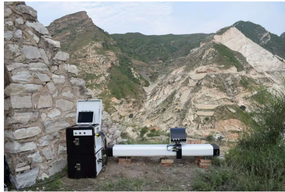
Figure 4. MPDMMR-LSA radar system.
