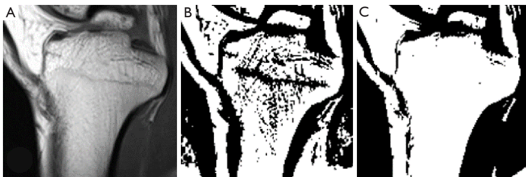
Figure 8 The adaptive thresholding with different sizes of the pixel neighborhood. (A) The original MRI image. (B) The binary image of 41 pixels neighborhood. (C) The binary image of 141 pixels neighborhood. MRI, magnetic resonance imaging.
