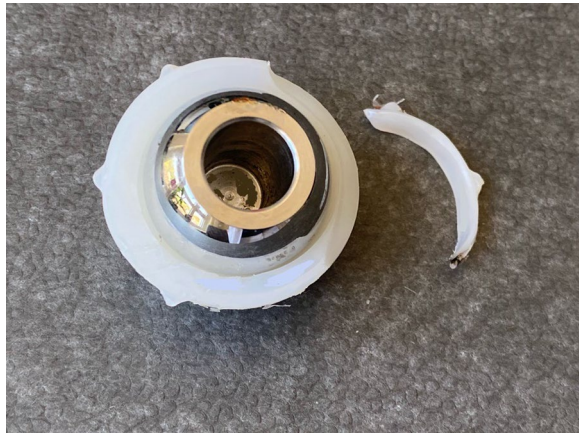
Fig. 5 In this particular case the replaced liner shows damage on one edge, with no signs of wear or ovalization. The image has been edited to obscure the serial numbers
