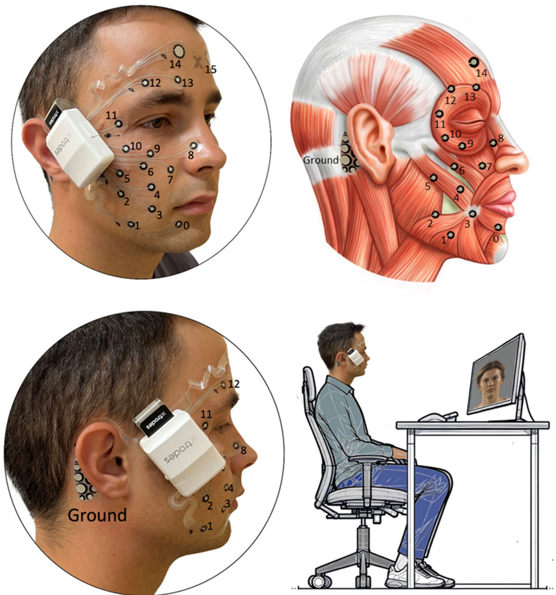
Figure 1. The experimental setup and the positions of the electrodes on the face: Channel 0–14 on the right side of the face and channel 15 on the contralateral left forehead. In addition, a reference electrode is placed on the right mastoid. Participants were sitting in front of a computer screen, followed the instructions of a video tutorial, and imitated the shown facial expressions (Illustration: courtesy of Sonja Burger).
