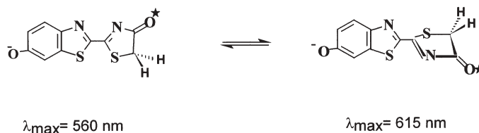
Figure 7. Mechanisms of bioluminescence color determination.
