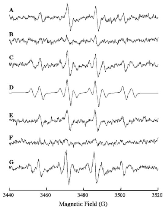
Figure 1 EPR analysis of O_2^{\bullet-} -scavenging activity of intact mitochondria
