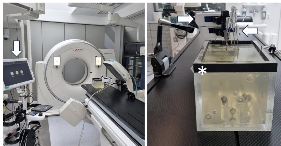
Figure 1. Experimental setup showing the phantom (*) centered below the C-arm. The robotic device consists of two parts: the lower positioning part (POS, ←) and the upper angulation part (ANG, →). The planning monitor (↓) can be operated via touchscreen.
