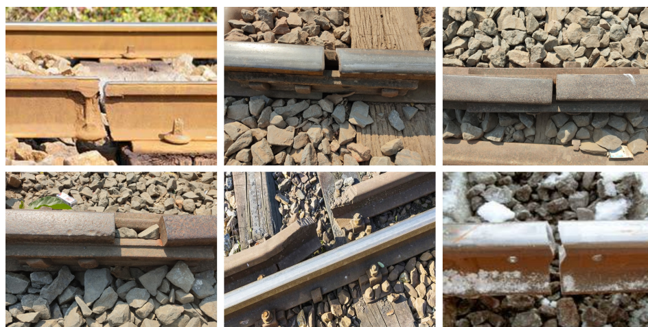
Figure 4. The sample images of railway tracks with faults (defect). The dataset consists of images of different views, including top and side views.
