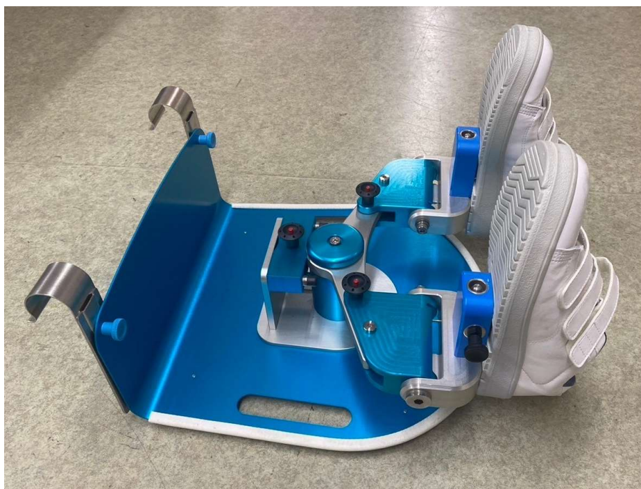
Figure 1. LEX, which comprises right and left pedals, shoes, a metal base, hooks, and a motion control mechanism. LEX: leg exercise apparatus.
