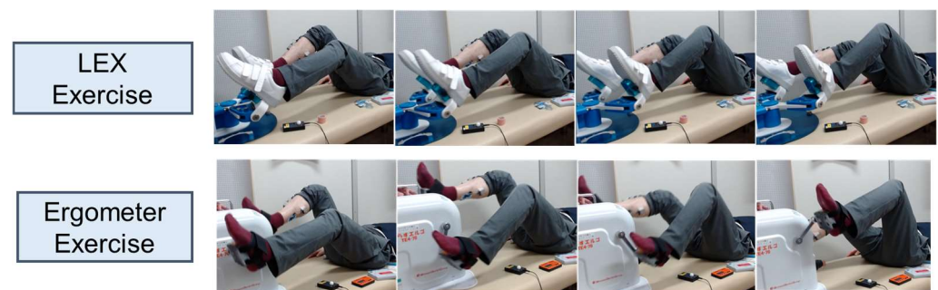
Figure 2. Illustrations depicting each exercise. The upper photos show the exercise with LEX and the lower photos show the exercise with an ergometer.
