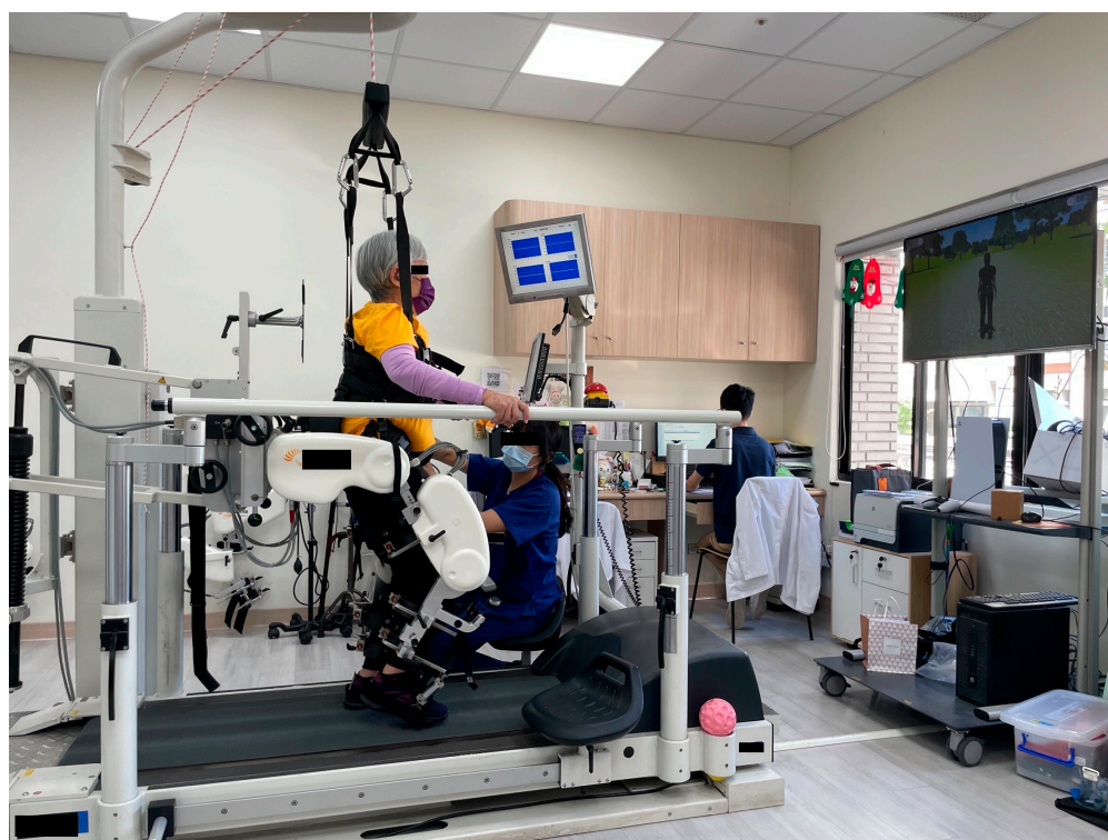
Figure 1. Robotic-assisted gait training (RAGT) device Lokomat. The patient is loaded onto Lokomat with the assistance of a trained physiotherapist. Augmented feedback with walking scenario provides increased attention and participation of the patient.
