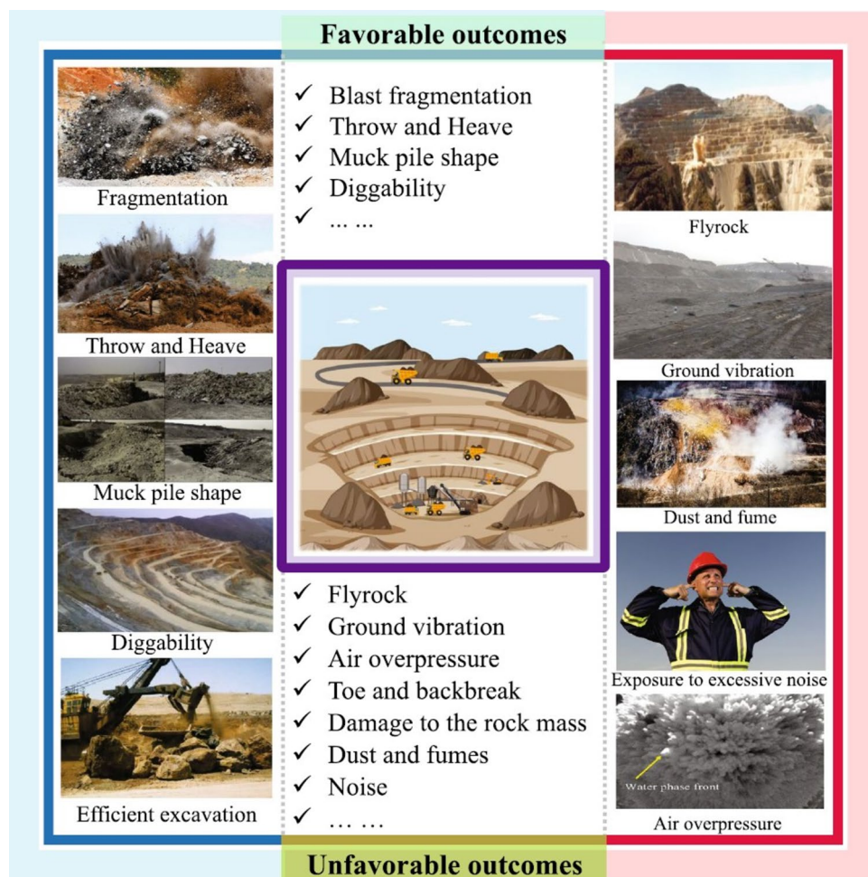
Fig. 1. The favourable and unfavourable outcomes of rock blasting (Source: 9 ).
