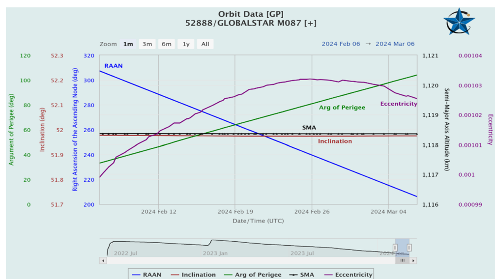
Figure 1. One-month projection for Globalstar satellite with orbit data including altitude (km), eccentricity, right ascension (deg), inclination (deg), argument of perigee (deg), and Date/Time on X-axis. Source: Celestrak.
