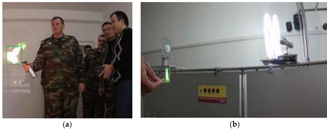
Figure 7. Footage of laboratory experiments: (a) recognized fire with a large flame; (b) recognized small size fire against the background of a fluorescent lamp.
