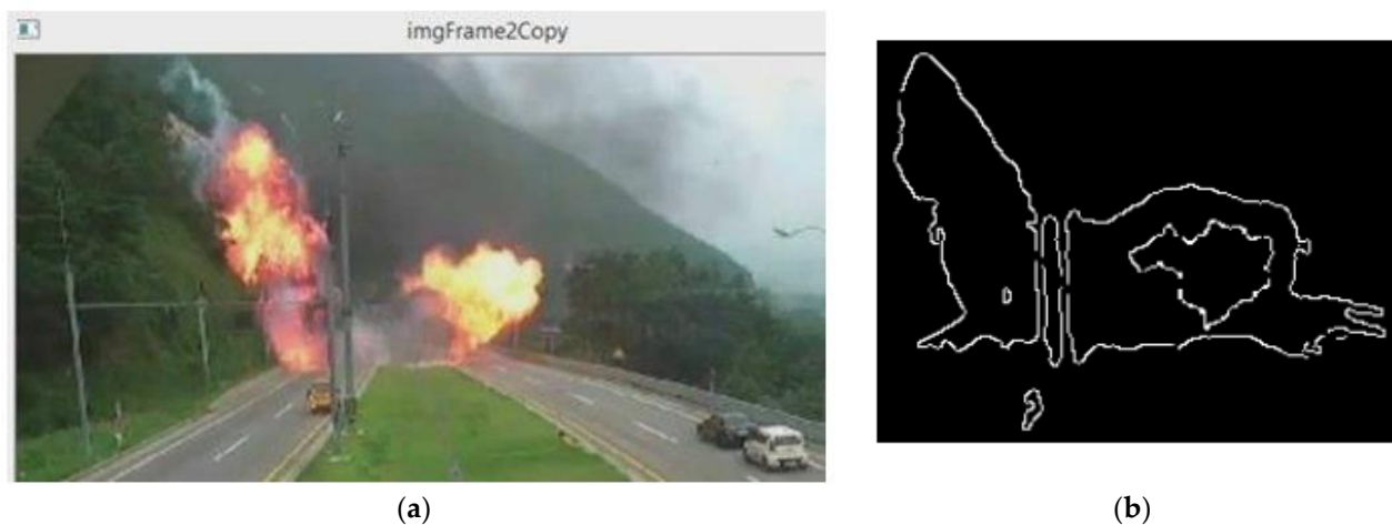
Figure 5. (a) Original input image; (b) Outline image of fire with two rings.
