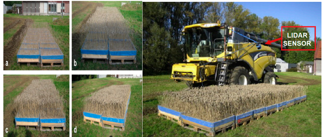
Figure 16. Different crop densities and combine harvester with LiDAR system (a) 100 ears per m^2 ; (b) 200 ears per m^2 ; (c) 300 ears per m^2 ; (d) 400 ears per m^2 [194].
