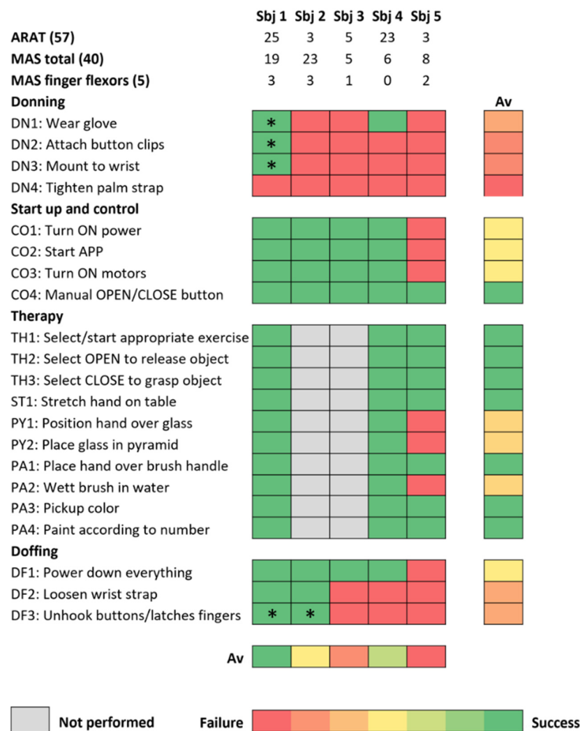
Figure 1. Checklist results represented as a heatmap. The results averaged over the subjects, and items are presented on the right and at the bottom of the heat map, respectively. The items “DN”, “CO”, and “DF” were evaluated during the assessments at S0 and S1, the other items only at S1. The tasks are ranked successful (1, green, i.e., no problem/issue in item completion without external intervention) or failed (0, red, i.e., failure and/or external intervention required to solve the item). Intermediate nuances between green and red are average values (Av) between 0 and 1 over subjects and items, respectively. DN: donning; CO: start-up and control; TH: all therapy exercises; ST: Stretching; PY: Pyramid; PA: Painting; *: item that could not be performed without external intervention before BoNT-A injections (S0) but could be performed after BoNT-A injections (S1).
