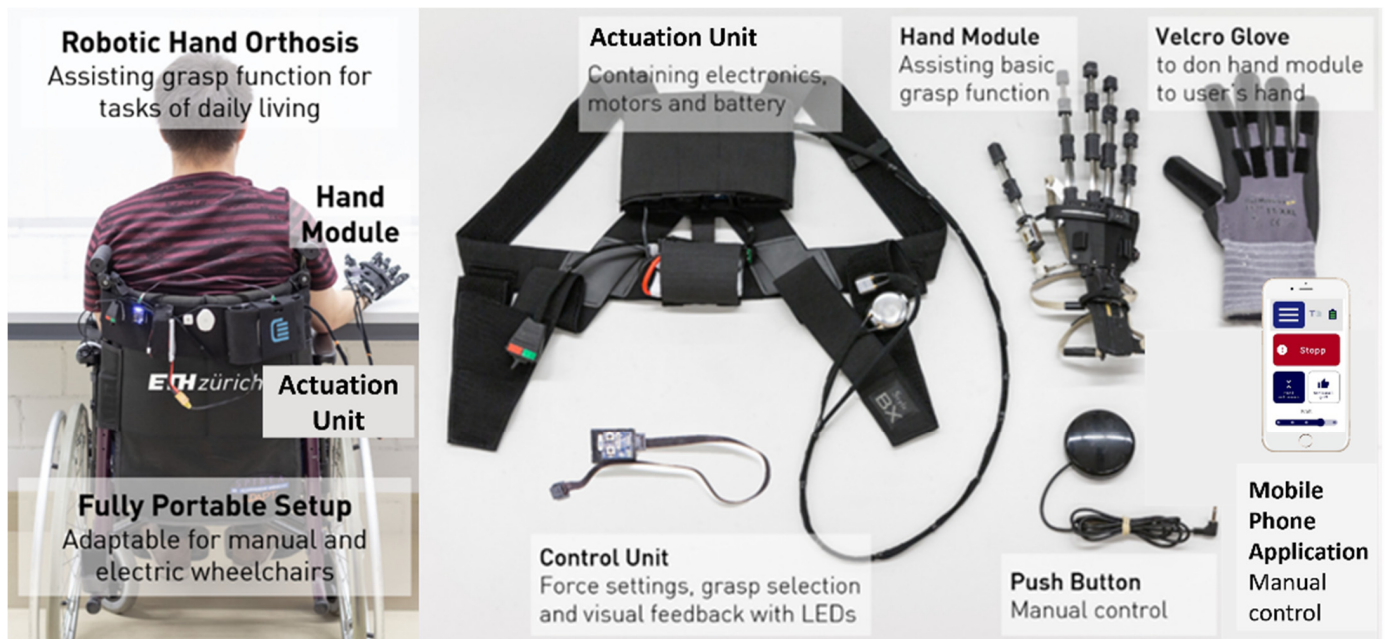
Figure 6. RELab tenoexo overview: the RELab tenoexo can be worn by the user or mounted on a wheelchair (left). The hand module (148 g) can be placed on a user's hand using a glove with Velcro and button-clips and is actuated by motors placed in the actuation unit (720 g) together with the electronics. Different intention detection strategies (e.g., push button, mobile phone application) can be used to trigger the motion of the RHO (right).
