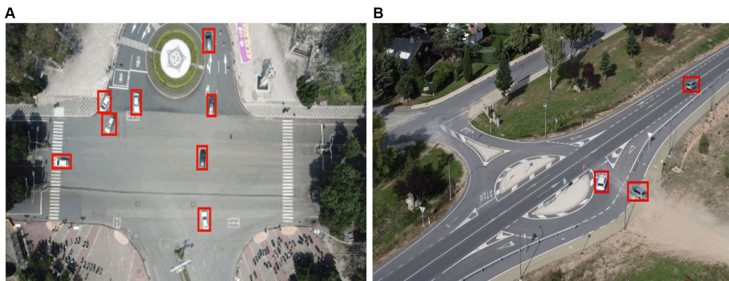
FIGURE 6 Vehicle Detection over (A) VEDAI and (B) SRTID datasets marked with red boxes via the YOLOv8 algorithm.
