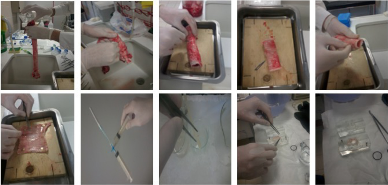
Figure 1. Stepwise demonstration of tracheal specimen preparation. Steps that demonstrate the sequence of sheep tracheal tissue handling, posterior tracheal membrane excision, and its treatment with Krebs's Ringer bicarbonate buffer or cigarette smoke extract (CSE). Using forceps, the intact membrane was mounted onto a Ussing chamber for trans-epithelial resistance recordings during exposure to Krebs's Ringer bicarbonate buffer or CSE complemented Krebs's Ringer bicarbonate buffer.
