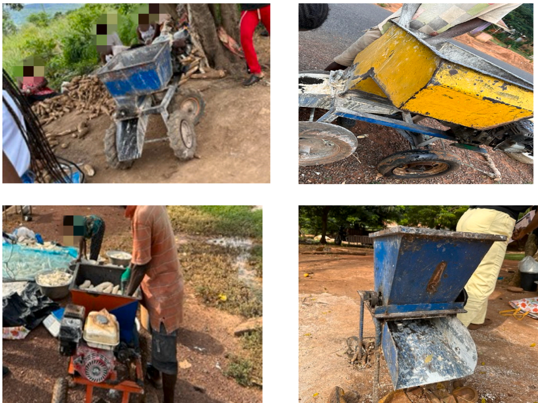
Fig. 2. Locally made cassava grater in Ghana.
