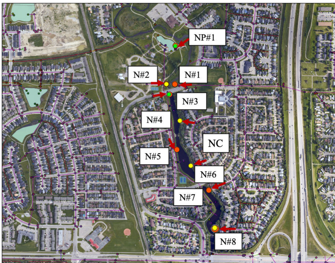
FIG 2 Map of human sewage marker (HF183) detection within stormwater outfalls into Nose Creek (NC) in Airdrie, Alberta, 2021. Note the overlaid colored dots representative of HF183 detection at quantifiable levels (red), detectable but not quantifiable (yellow), and not detected (green) in the Nose Creek Pond (NP#1) and Nose Creek sites (NC#1–8). Red arrows represent the directional flow of stormwater. Note that all maps presented were created and co-owned with the City of Airdrie, and have been used with permission.
