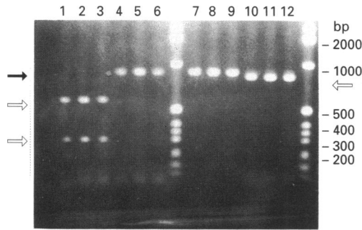
Figure 1 Specificity of amplification of genomic DNA using sense primer Nat-Hu20 with either Nat-Hu21 or Nat-Hu22 as anti-sense primer
