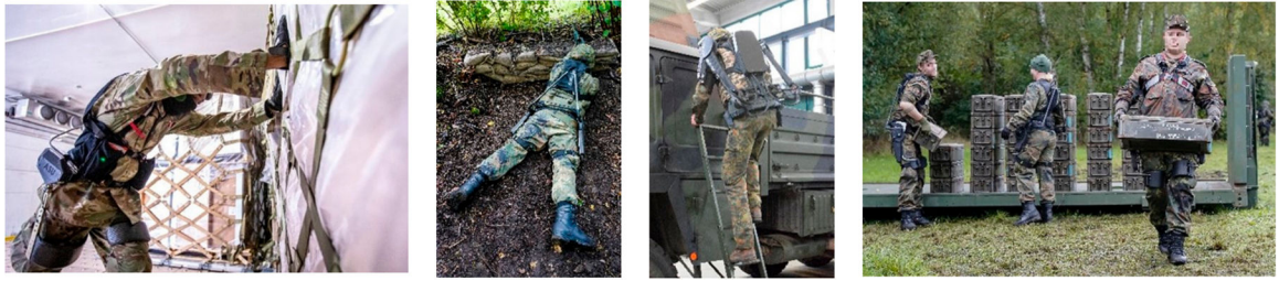
Figure 2. Wearable robots for occupational military activities. From left to right: Aerial Porter pushing large pallets, a soldier with exoskeleton kneeling on the ground in a defensive position, a soldier climbing a ladder with an exoskeleton, and soldiers transporting heavy boxes with an exoskeleton support them during lifting.
