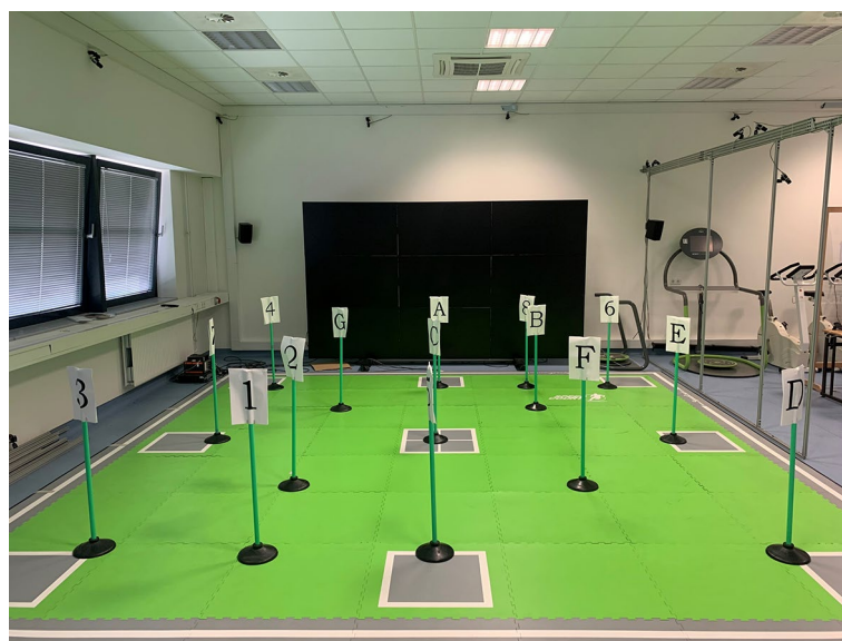
Fig. 2. Experimental set-up of the “Trail-Walking-Test”. The participants had to walk towards the cones in an alternately ascending order (1, A, 2, B, 3, C and so on).
