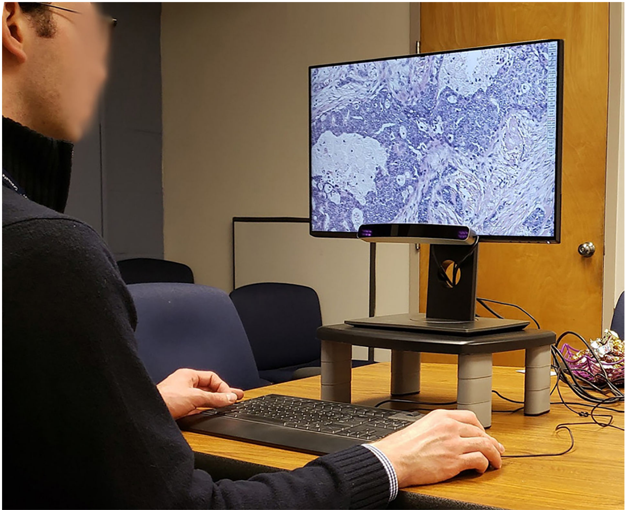
Figure 2. A pathology trainee (face blurred for privacy) interpreting a WSI during the study; the eye tracker is attached to the bottom of the computer monitor, and the trainee is navigating the zoomed case using the computer mouse.
