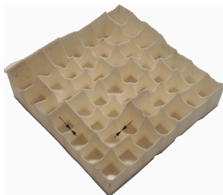
Figure 8. Location of measuring points for calculation of minimal thickness for successful injection molding.
