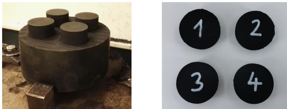
Figure 2. The sampled specimens and their location within the rubber product.
