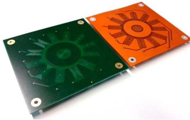
Figure 15. Rigid (left) and flexible (right) PCB-based eddy current sensor array [254].
