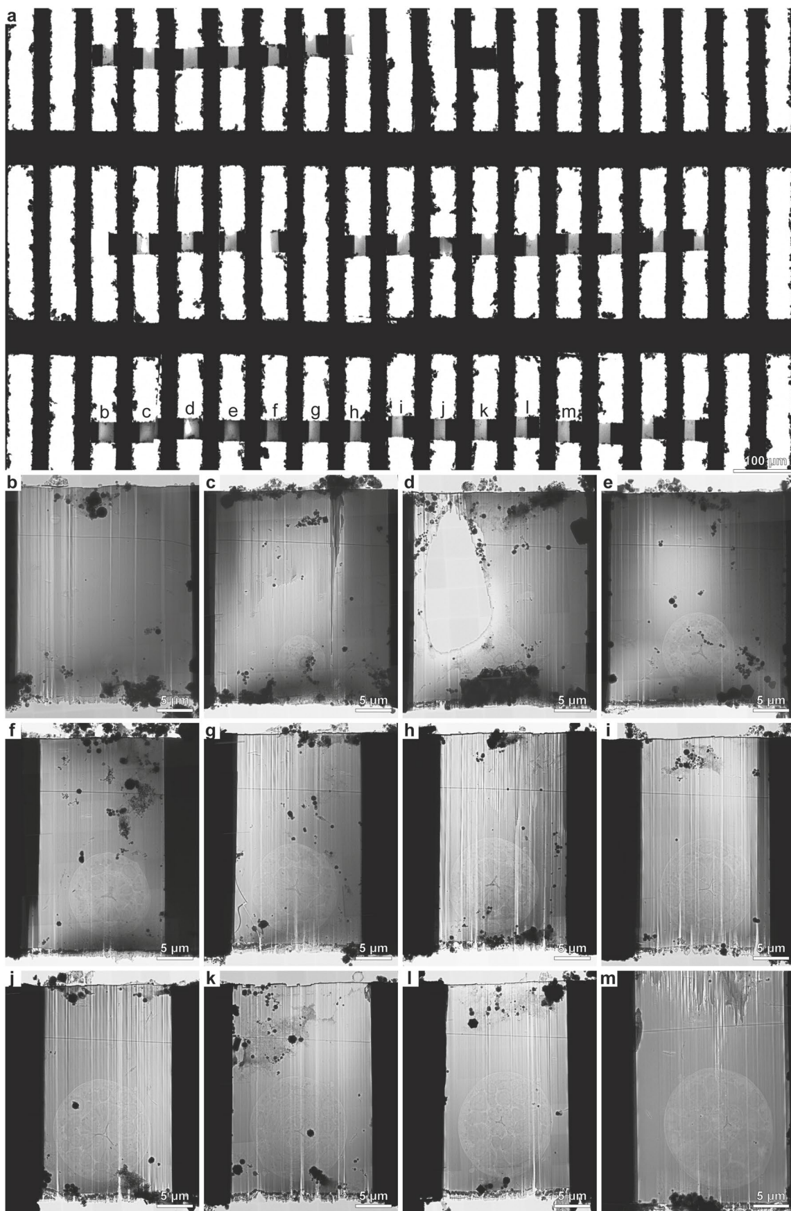
Extended Data Fig. 6 | TEM overview of the grid derived from the double-sided attachment Serial Lift-Out experiment. a , TEM low magnification overview image (magnification 125 \times ) of the lamella region of the Serial Lift-Out receiver grid for double-sided attachment. b-m , Lamella overviews
