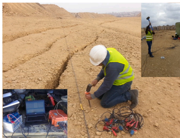
Fig. 17. Seismic data acquisition for P-wave seismic velocity using the 14Hz geophones and 10 kg sledgehammer taken in the sliding area at the eastern part of the study area.
