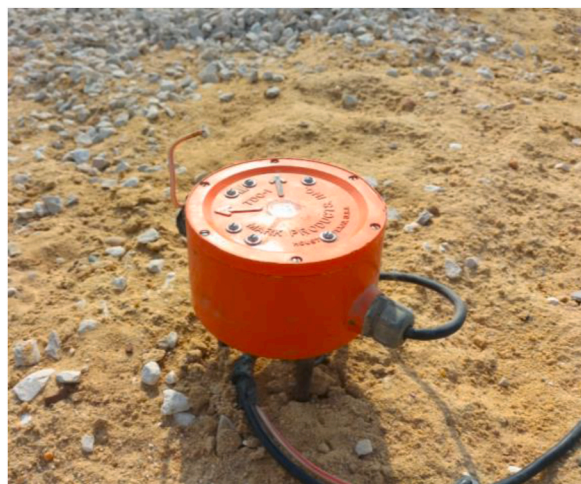
Fig. 19. Triaxial geophone 4Hz was used to collect microtremors data in this study.
