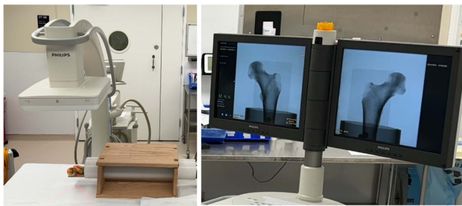
Figure 1. Experimental Setup: The cadaveric bone specimen was positioned on a radiographic table in a manufactured rotation device made of a radiopaque plastic pipe and a box. A C-arm fluoroscopy machine (Phillips Zendition 70, Eindhoven, NL) was centered 12 inches above the femoral head for imaging of the Lesser Trochanter (LT) profile. Observers rotated the pipe at the distal end to adjust rotation angle of the bone until they were satisfied that they had matched the reference image.
