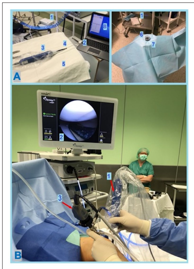
Figure 1. Electromechanical evaluation during knee arthroscopic surgery. (A) Preparation for electromechanical measurements. (1) Arthro-BST electrical isolation box. (2) Laptop computer. (3) Arthro-BST handle. (4) Sterile tip with electrodes. (5) Sterile table. (6) Sterile container with saline. (7) Sterile-covered ultrasound bath. (8) Arthro-BST software. (B) Electromechanical assessment during arthroscopy. (1) Sterile draped Arthro-BST handle with attached tip. (2) Sterile tip with electrodes at the measurement site of medial femoral condyle weight-bearing surface. (3) Regular arthroscopic camera.
