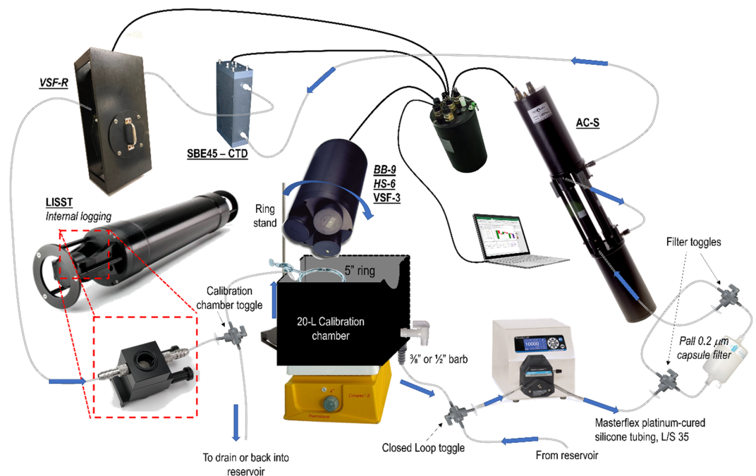
Fig. 1 Schematic of in-line sampling apparatus for inherent optical properties of phytoplankton cultures.
