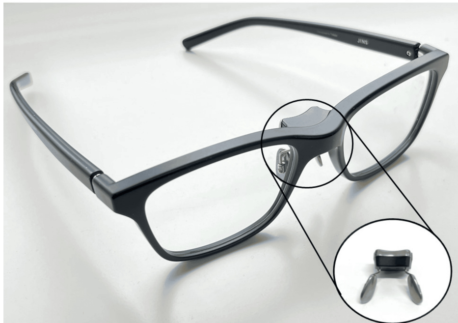
FIGURE 1: The JINS MEME with a built-in gyroscope and acceleration sensor electrodes
