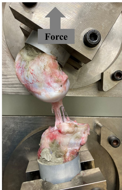
FIGURE 3 Biomechanical evaluation of the femur–graft–tibia (FGT) complex. The FGT complex was mounted on a tensile tester using a set of specially designed grips. A tensile load was then applied to the grafted tendon parallel to its long axis. Cyclic testing was performed initially to simulate the tibial anterior drawer setting, followed by tensile testing. Failure modes were recorded. The structural properties (upper yield load, maximum load, linear stiffness and elongation at failure) of the complex were determined through software calculations.
