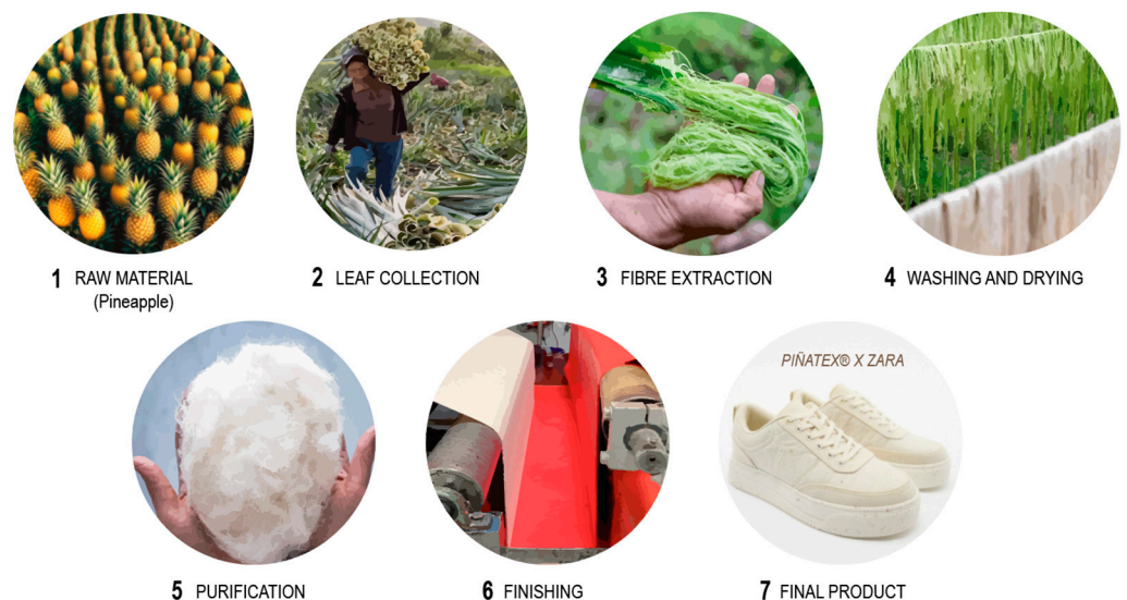
Figure 9. The Manufacturing Process of Piñatex.
