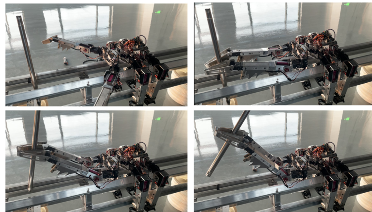
Figure 8. Robot gripping rod part experiment.
