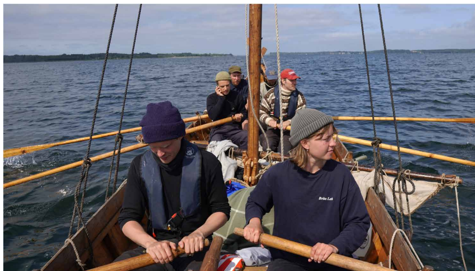
Fig. 3. Experimental insights into Greenland Norse seafaring capabilities: example of a "smaller" vessel (with oars and sail). This is a Norwegian fying during sea trials. Note the very limited space for cargo (Roskilde Fjord, Denmark, June 2023). Photo: G.J.
