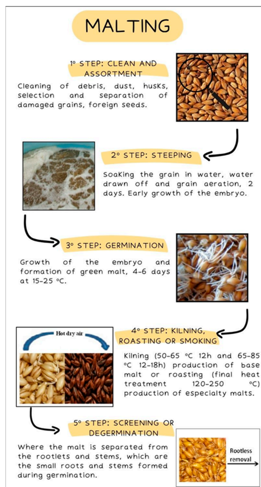
Figure 6. Illustration of main steps involved in the malting process, key events, conditions for occurrence, and objectives.
