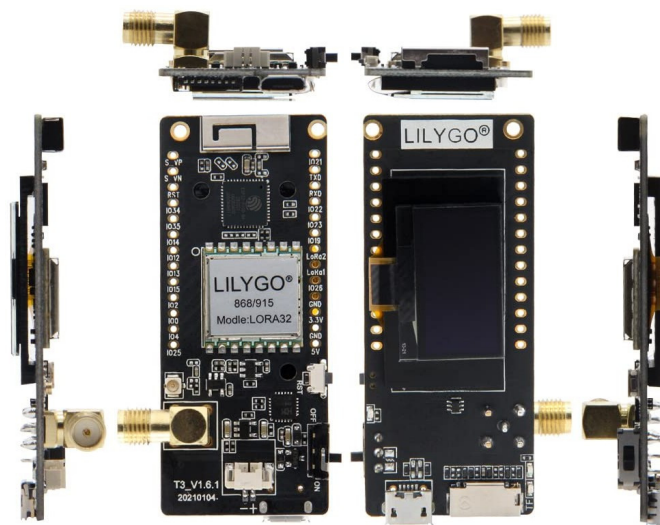
Figure 7. Top (right) and bottom (left) view of the Lilygo LoRa32 device (Source: [61]).
