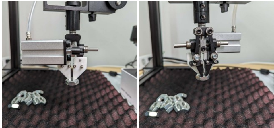
Figure 3. Grippers designed for nut grasping.
