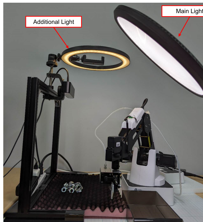
Figure 18. Experimental setup with additional lighting source. In addition to the existing lighting conditions, we introduced an additional light source. Furthermore, we altered the color of this additional light to provide a variation from the training environment. The lux level was increased to 1500.
