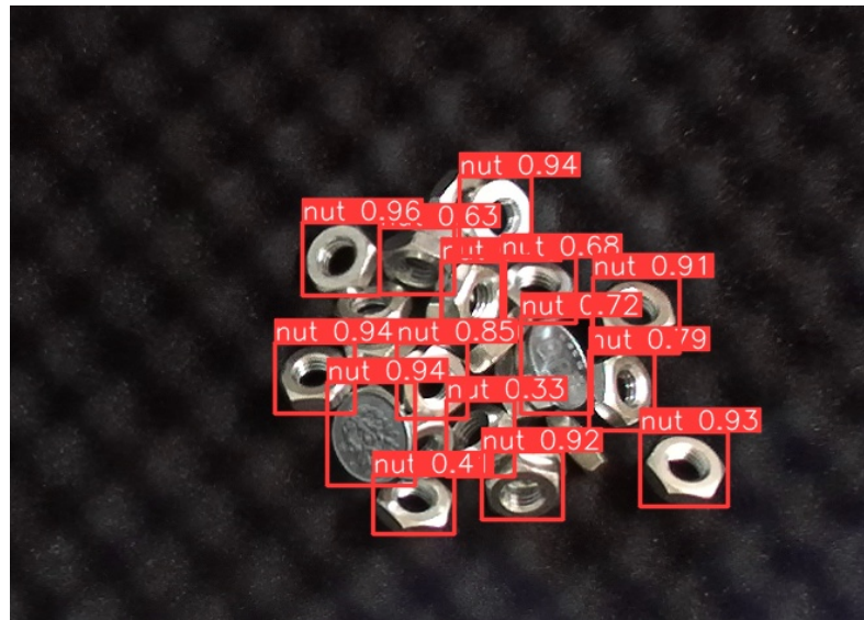
Figure 21. YOLO's detection results with 100-yen coin. Coins were mistakenly identified as nuts, with confidence scores exceeding 0.90, even higher than those for actual nuts. Additionally, for some nuts, the model failed to achieve a confidence score above the 0.5 threshold.
