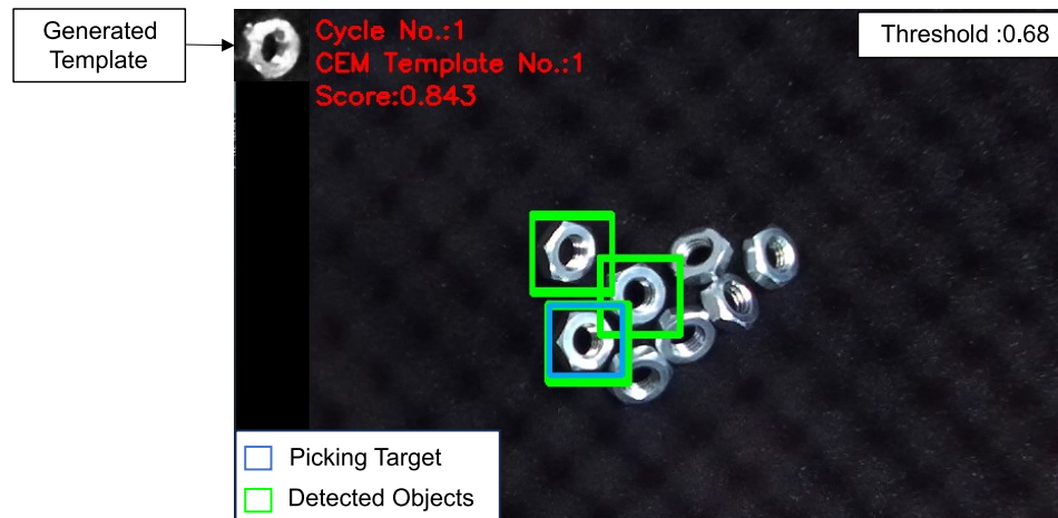
Figure 8. Generated template and its matching result. The green windows indicate the detected objects with a matching score above the threshold of 0.68. Meanwhile, the blue window highlights the location with the highest matching score, serving as the picking target for the robot.
