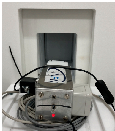
Figure 10. The MiniRadMeter placed on a tray in front of the neutron generator output window.
