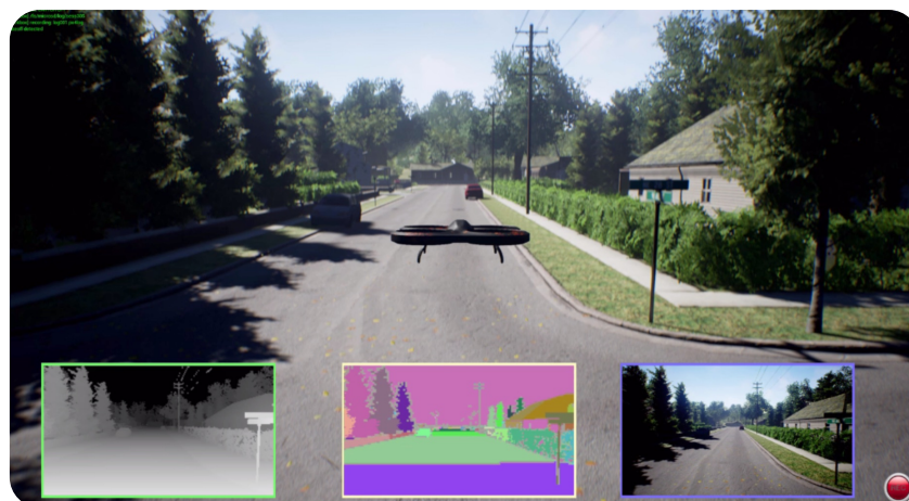
Figure 3. AirSim with an aerial vehicle in an urban environment [13,14].
