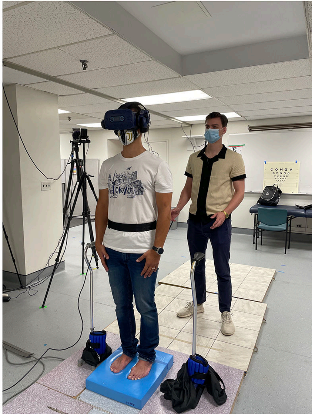
Fig. 1: Experimental setup: A participant is standing on foam placed on top of a force-platform while wearing the HTC Vive headset.
