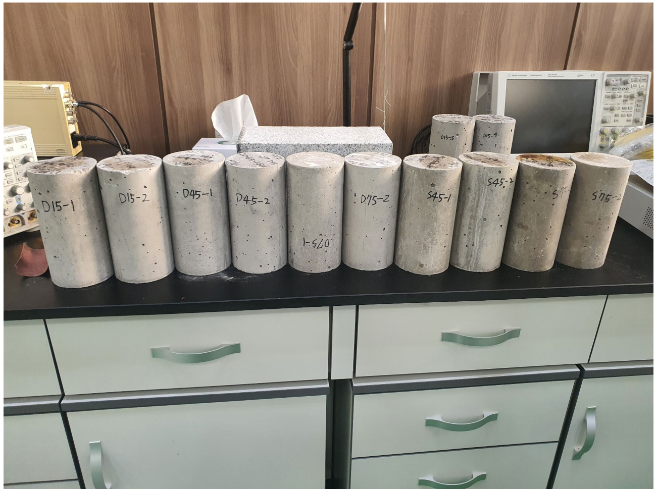
Fig. 6. Concrete specimens for verification.
