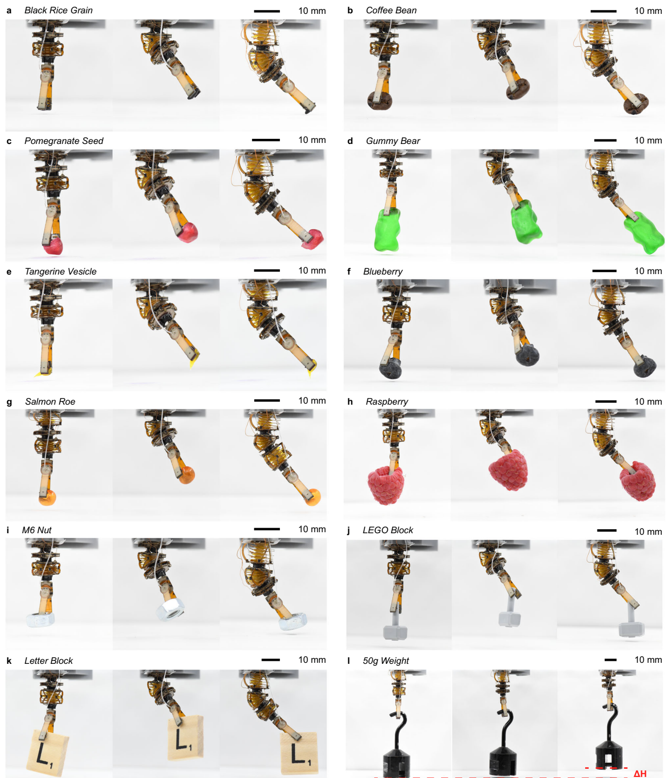
Fig. 7 | SHY robotic manipulator performing pick-and-place tasks. Objects (soft and hard) included in the pick-and-place test are as follows. a A black rice grain. b A coffee bean. c A pomegranate seed. a–c demonstrate the robot can manipulate small objects. d A gummy bear. e A tangerine vesicle. f A blueberry. g A salmon roe.
