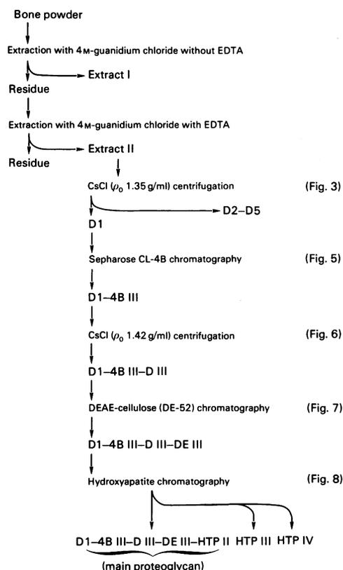
Scheme 1. Flow diagram showing the steps in purifying the bone proteoglycans. For full experimental details see the Materials and methods section.
