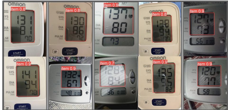
Fig 7. Examples of LCD detection results on images captured from Omron M7 and Omron 3 devices.
